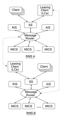
**Figure 6:** Networking the RMSs using the leasing client.
