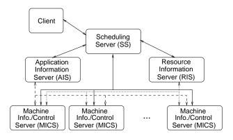
Figure 1: Architectural block diagram of the RMS.
